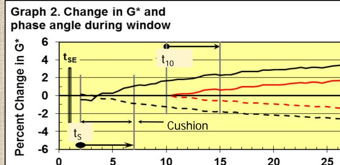
$t_{TT}$  – time zero, DSR indicates target temperature  $\pm 0.1^{\circ}C$   $t_{SE}$  – time when specimen is at thermal equilibrium  $t_{C}$  – cushion between equilibrium and start time  $t_{S}$ ,  $t_{E}$  – time at start an end of test window  $t_{10}$  – 10 minute wait time as per AASHTO 315, ASTM 7125
